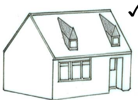
Size and position of dormers subordinate to main roof and related to ground floor openings
